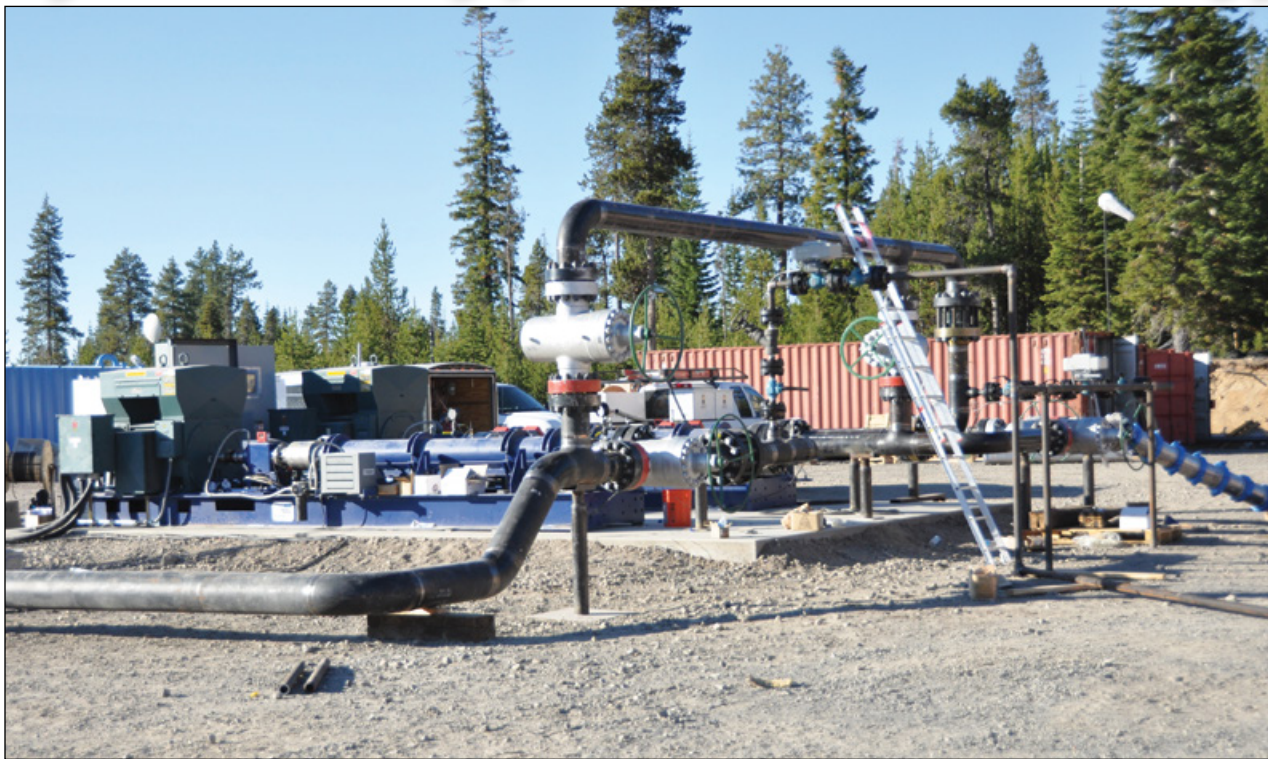
AltaRock utilizes high-pressure multi-stage pumps engineered specifically for stimulation to induce hydroshearing and increase permeability in both traditional hydrothermal and EGS wells.
