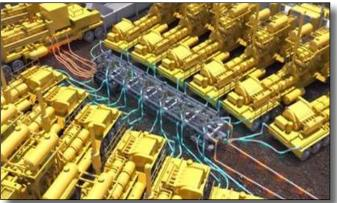
piped directly into the Pressure Exchanger at relatively low pressures instead of into frac truck pumps. Simultaneously, the frac pumps are used only to pump high pressure water into the exchanger.
